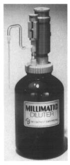
• Tri-Continental Scientific's Millimatic Diluter couples a factory-calibrated, 140-position diluent assembly with a wide range sampling unit to make laboratory dilutions easier. Sample and diluent plungers are Telfon-coated for bind-free operations. Diluent volumes: 1 to 15 ml, in precalibrated 0.1 ml increments. Details: Tri-Continent Scientific Inc., 12933 Lakeshore North, Auburn, CA 95603.
